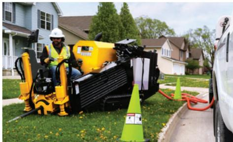
**COMPACT BUT POWERFUL.** The D10x15 S3 stands out due to its compact design and light weight. With 10,000 lb (44.5 kN) of thrust/pullback and 1500 ft-lb (2033.7 Nm) of rotational torque, it has the power required for tough ground conditions and pulling reamers.
