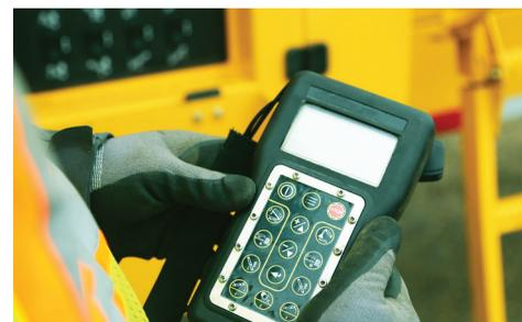
**CONVENIENT CONTROL.** Operators can control the machine through either the machine display mounted on the control panel, or through a transceiver remote. From either control, the operator can choose from four programmable presets or adjust on the fly based on incoming material.
