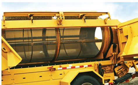
**DRUM SERVICE ACCESS.** A set of dual-hinged doors on both sides provide convenient access to the full length of the trommel drum from ground level for drum service and removal.
