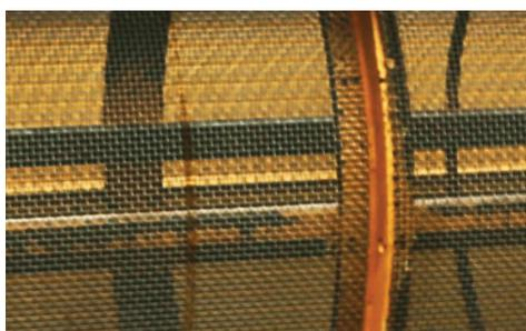
**PRODUCT VARIETY.** Change product sizing more efficiently with the quick-change screen design. Five large bolts adjust a tensioning hook to allow operators to quickly change screen sizes.
