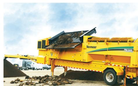
**GRIZZLY SCREEN OPTION.** The optional grizzly attachment can be mounted over the hopper to prescreen large materials and create more consistent overs material.
