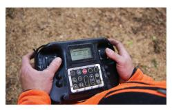
**OPTIONAL REMOTE CONTROL.** An optional remote control allows operators to maneuver the stump cutter while away from the unit. The joysticks help to increase operator control and comfort.
