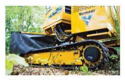
**ZERO TURNING RADIUS.** The planetary traction drive helps provide traction while the counter-rotating tracks provide tight maneuvering in difficult jobsite conditions.
