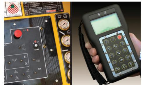
**CONVENIENT CONTROL.** Monitor real-time performance and data via the on-rig display or remote control.
