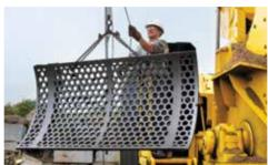
SIMPLE SCREEN CHANGES. Operators can change product sizes easily with the onboard screen handler system, offering a mechanical or optional air operated hoist assembly.
